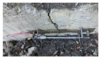
Model EDJ-40V Crack meter installed
